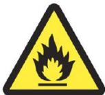
Freezer and refrigerators that use flammable refrigerants are marked with this specific triangle symbol that notifies the servicer of the presence of flammable refrigerants. The symbol is located on the compressor and unit nameplate.
