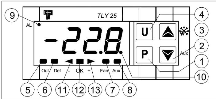
**1 - Key P** : Used for setting the Set point and for programming the function parameters
