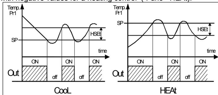
In the event of cell probe error (Pr1), it is possible to set the instrument so that the output "Out" continues to work in cycles according to the times programmed in the parameter "tonE" (activation time) and "toFE" (deactivation time).
