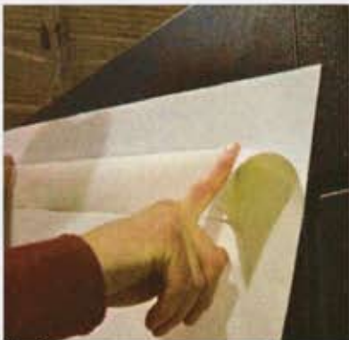
Step 1 Peel and fold backing paper from decal about 2" down from top.
