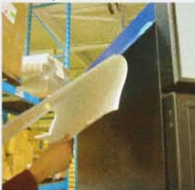
Step 4 Lift up decal and peel about 6 inches of backing paper from decal.
