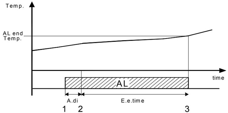
Note: If the power fails during an alarm from a digital input, the instrument records the duration of the alarm up until the moment the power failure began.
