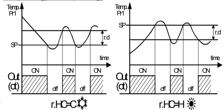
As regards the operating mode programmed in the "r.HC" parameter, the regulator automatically assumes that the differential has positive values for a Refrigeration control ("r.HC"=C), negative values for the Heating control ("r.HC"=H).
