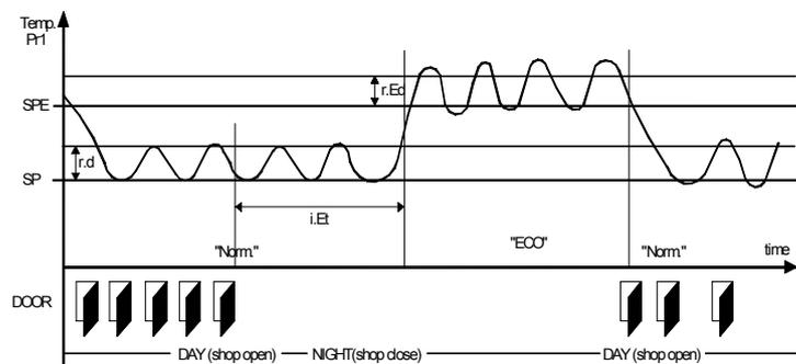
Example of automatic switching between Eco mode and normal mode. During working hours the door is frequently opened and the controller stays in normal mode. When the door has not been opened for time "i.Et", the controller switches to Eco mode. As soon as the door is opened again, the controller reverts to normal mode.
