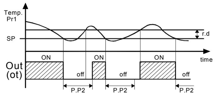
Third control (par. "P.P3") foresees an inhibition to the activation of the output "Out" by a time delay that starts when the output was turning on last time (delay between switching-on).
