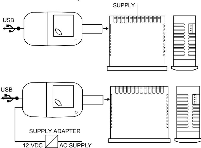
The same device can connect the instrument via USB to a PC and through the proper configuration software tools "TECNOLOGIC UniversalConf", it's possible to configure the operating parameters. To use the device A01 it's necessary that the device or instrument are being supplied.
