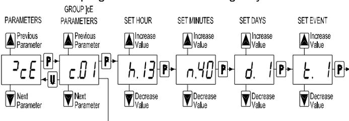
After selecting the desired parameter, press the P key repeatedly to cycle through the following:
