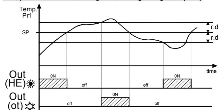
If the parameter "r.HC" is programmed such that "r.HC" = nr the output configured as "ot" operates with a cooling action (as "r.HC" = C) whereas the output configured as "HE" operates with a heating action. In this case the regulating set point for both outputs is whichever of SP, SPE and SPH is active, and the intervention differential ("r.d" or "r.Ed" or "r.Hd") is automatically assumed by the regulator to have positive values for the cooling action, negative values for the heating action.
