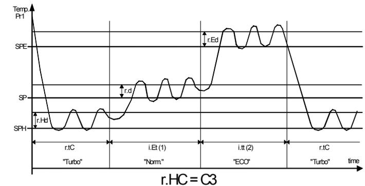
(1) - The time i.Et is reset every time the door is opened and in the case shown the door is always closed.
