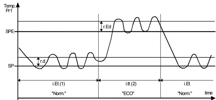
(1) - The time i.Et is reset every time the door is opened. In the case shown, the door is always closed.
