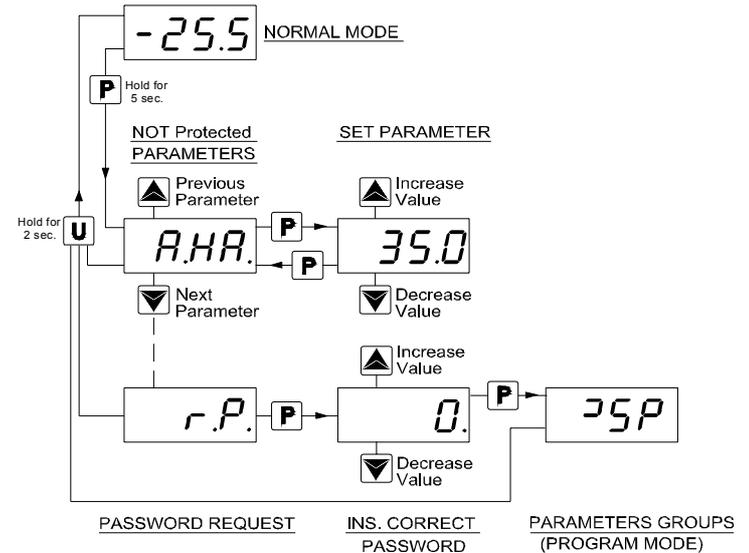
With regard to setting unprotected parameters, an exception is HACCP alarm-related parameters ("H.01", "H.02", etc. which are visible only when there are alarms stored in memory) whose display level can be set via the "t.HA" parameter.
