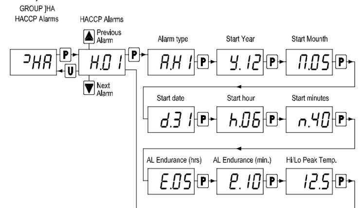
The instrument automatically sorts these parameters from most recent (H.01) to oldest (H.10) whenever an alarm is recorded or deleted.
