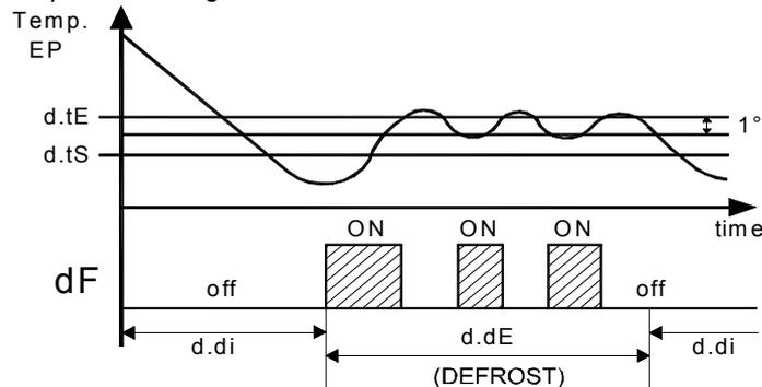
**Example of electric defrost with evaporator temperature control:** The defrost end after "d.dE" programmed time. During defrost the "dF" output switch on/off to control evaporator temperature in heating mode with set point "d.tE" and 1° differential (Hysteresis).
