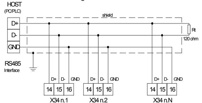
The interface circuit allows the connection of up to 32 instruments on the same line.
