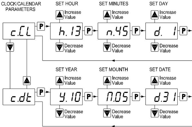
After selecting the "c.CL" parameter, press the P key repeatedly to cycle through the following in the order shown:
