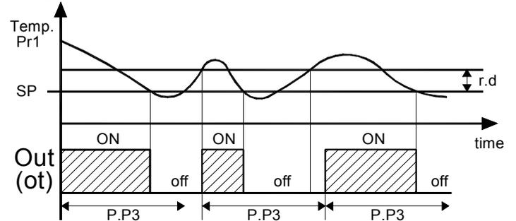
During the output inhibition the led OUT (Cool o Heat) blinking. It is also possible to prevent activation of the output after the instrument is turned on, for the time set in the parameter "P.od". During the power on delay phase, the display shows the indication od, alternating with the normal visualisation. All the functions are disabled by relative parameters = 0F.
