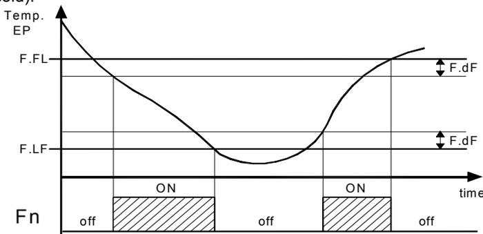
Notes: It is necessary to pay attention to the correct use of this fans temperature control functions because in the typical application of refrigeration the stop of the fans evaporator stops thermal exchange.
